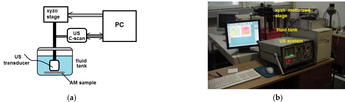
Figure 3. Ultrasonic equipment: (a) schematic diagram; (b) MicroSonic—Mark IV device.
