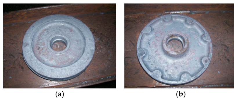
Figure 1. Half dies for obtaining wagon wheels: (a) upper half die; (b) lower half die.
