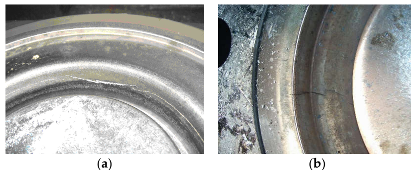
Figure 3. Defects arising in exploitation: (a) exfoliation, oxides, erosion; (b) cracks.
