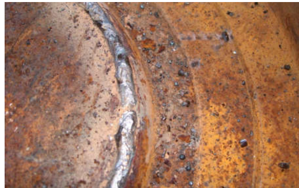
Figure 7. Half die reconditioned by loading with the experimental electrode.
