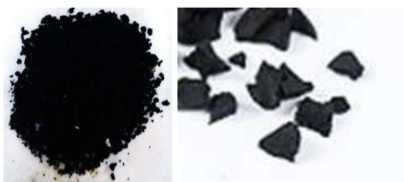
Figure 2. Sample of crumb rubber with sizes between 2 mm and 4 mm used in the present research as filler for the new composites.
