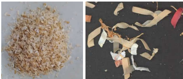
Figure 1. Sample of ABS shavings resulted in the furniture manufacturing process of edge banding melamine faced particleboard and used in the present research as matrix for new composites.
