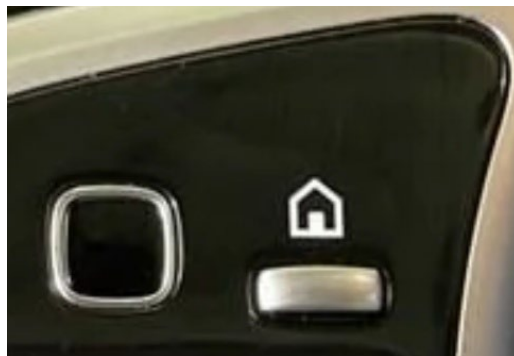
Figure 11. Laser engraving of the parts.
