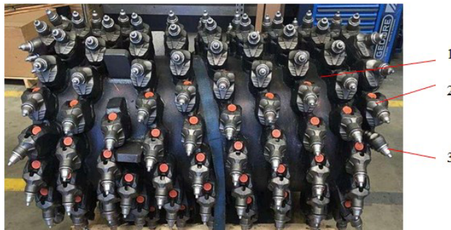
Fig. 2. Road structure milling drum: 1 - drum, 2 - milling tooth, 3 - mounting base.
