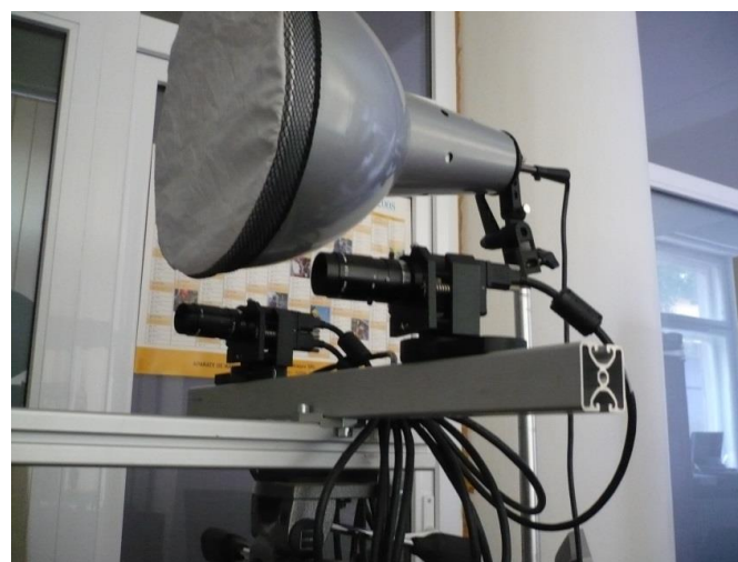
Figure 5. The Video Image Correlation (VIC)-3D setup.
