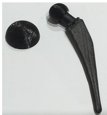
Figure 13. Hip endo-prosthesis after gluing the carbon fiber over the ABS plastic core [1].
