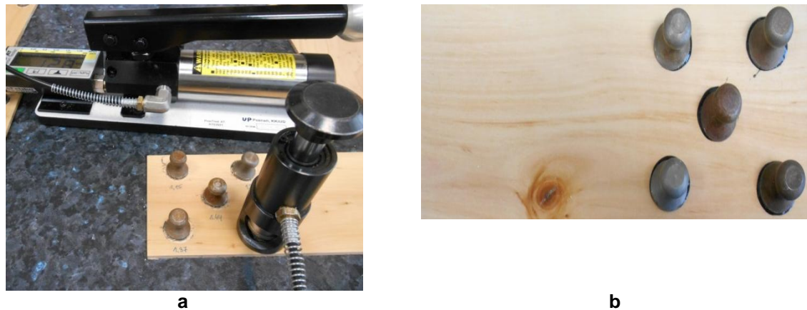
Fig. 4. PosiTest adhesion tester in action (a); dollicies glued on the sample (b)[16]
