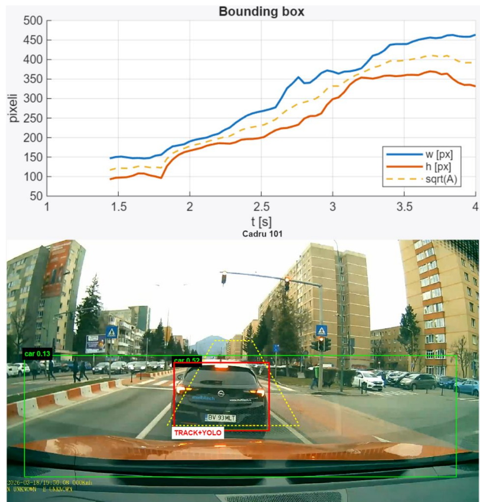
Figure 5. Example of temporal evolution of bounding-box dimensions during target approach (up) and vehicle YOLO detection during analysis (down).
