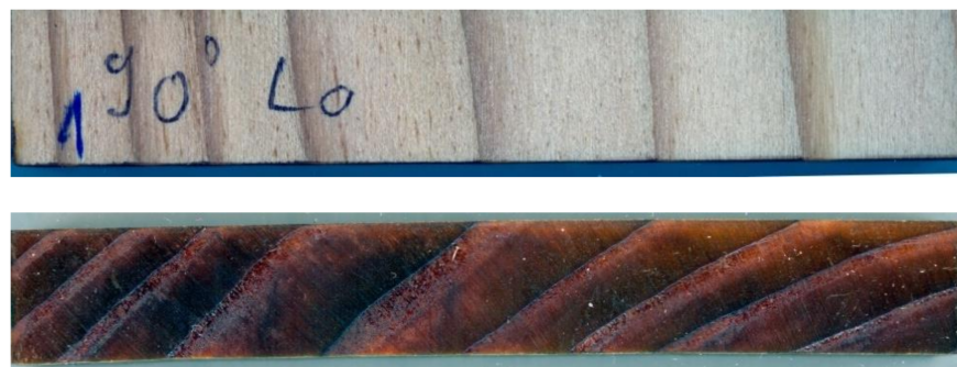
Figure 12. Larch processed by laser at 90° angle as relate to the grain (face-top image and cut edge—bottom image).
