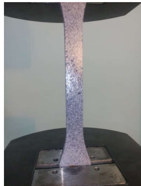
Figure 2. Tensile specimen clamped in tensile machine
