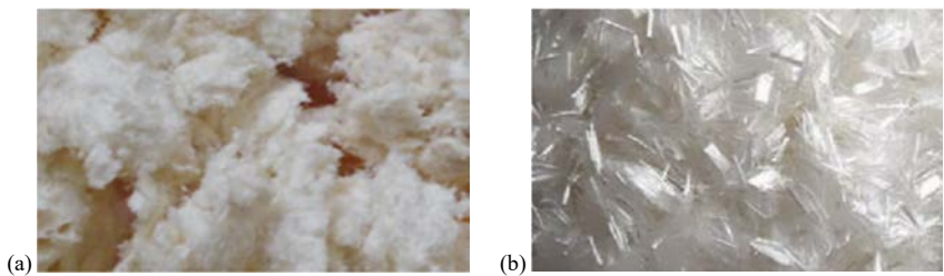
Fig. 1. Reinforcing materials: a) kevlar pulp; b) glass fiber chopped.
