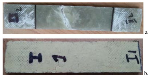
Fig. 4. The specimens after tensile testing: (a) glass fiber chopped reinforced epoxy resin composites; (b) kevlar pulp reinforced epoxy resin composites
