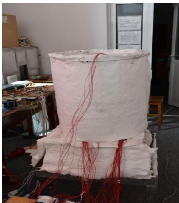
Figure 6. Heating stand, together with the thermal protection enclosure of the column [12].
