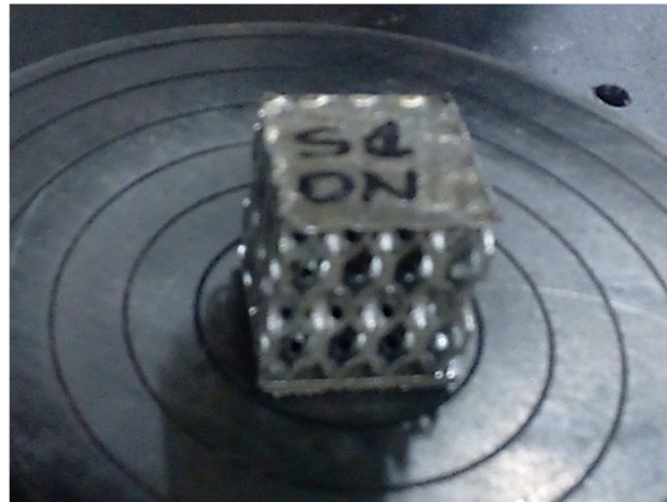
Figure 6. Compression testing of the sample with hyperbolical stiffness.
