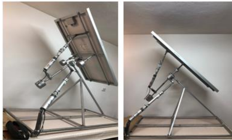
Figure 29. Physical prototype of the equatorial dual-axis tracking system.
