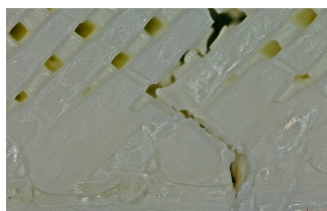
(b) Detailed fracture top view
