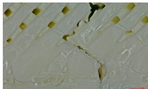
(a) Fracture view from above
