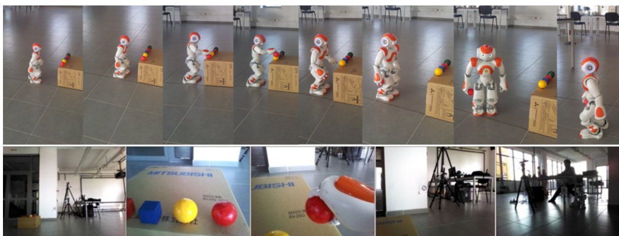
Figure 11. (a) NAO walks in the indicated direction, identifies the red ball, grabs it and returns to the user; b) the robot's line of sight viewed from different positions
