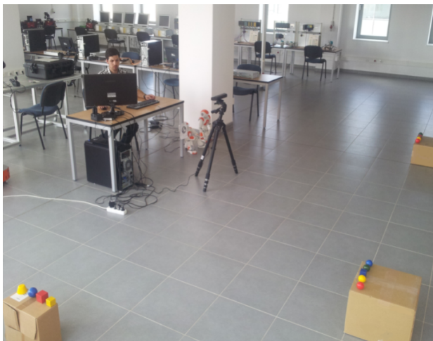
Figure 10. The operator sits in front of the Kinect sensor. He points at one of the three boxes and asks the robot to bring him a coloured object.
