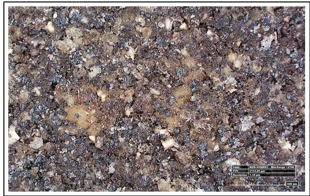
Figure 7. Surface appearance for the composite with bentonite matrix reinforced with \text{Al}_2\text{O}_3 and Fe particles.
