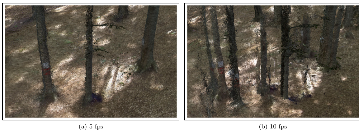
Fig. 4. Quality comparison between a point cloud generated with (a) 5 frames per second (fps) and (b) 10 fps. The snippets shown in (a) and (b) were captured from the same viewpoint. Except for the difference in the frame rates, the two point clouds were generated with the same settings. Using 10 fps resulted in an incorrect stem reconstruction, making the same tree appear several times in the point cloud.
