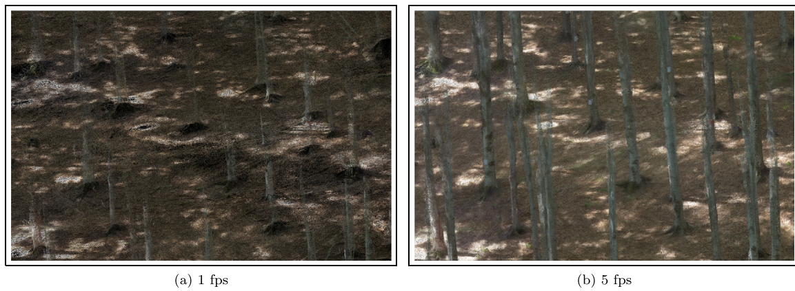
Fig. 3. Quality comparison between a point cloud generated using our videogrammetric approach with (a) 1 frame per second (fps) and (b) 5 fps. The snippets shown in (a) and (b) were captured from the same viewpoint. Except for the difference in the frame rates, the two point clouds were generated with the same settings. A larger number of video frames (5 fps) results in a higher level of detail in the point cloud.
