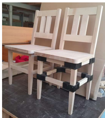
Figure 6. The two types of chairs subjected to final tests (experimental chair with 3D printed connectors on the right, and the reference one on the left).
