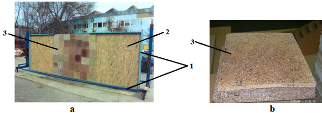
Fig. 1. Acoustic barrier: (a) experimental stand; (b) composite plate made from ABS chips.
