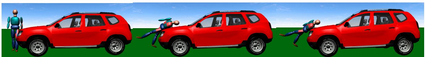
Figure 10. Example of collision for CSUV vehicle, at 5 m/s speed.
