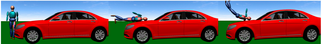
Figure 13. Impact phases for executive class vehicle.
