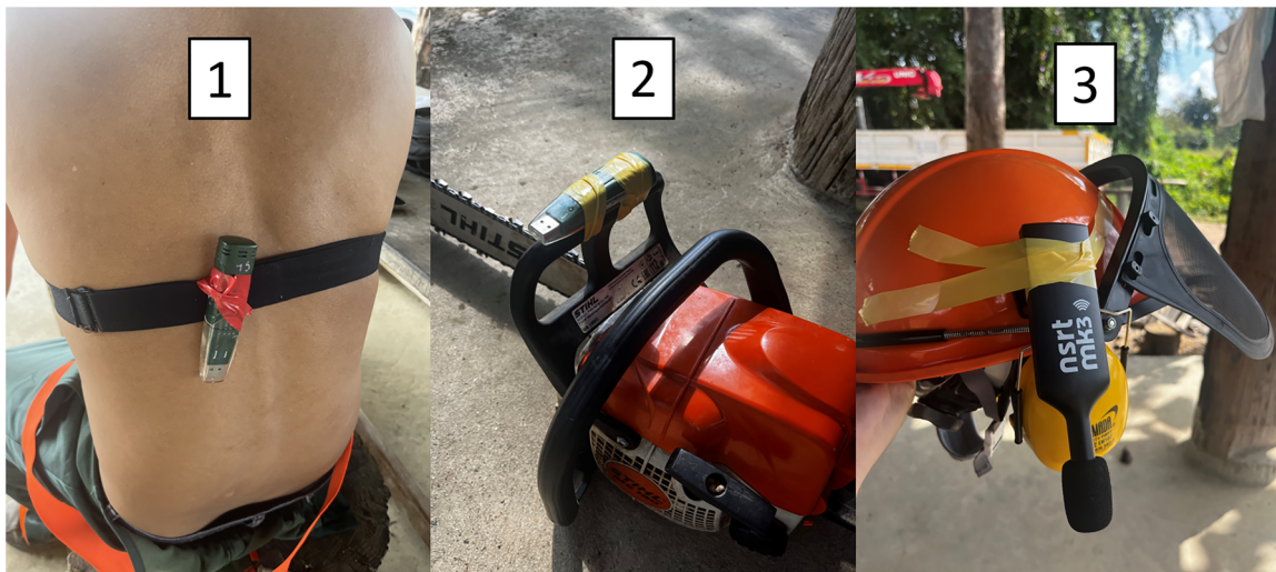
Figure 2. Instrumentation of data collection: triaxial accelerometers placed on operator's back (1) and chainsaw (2), and sound pressure meter on helmet (3).
