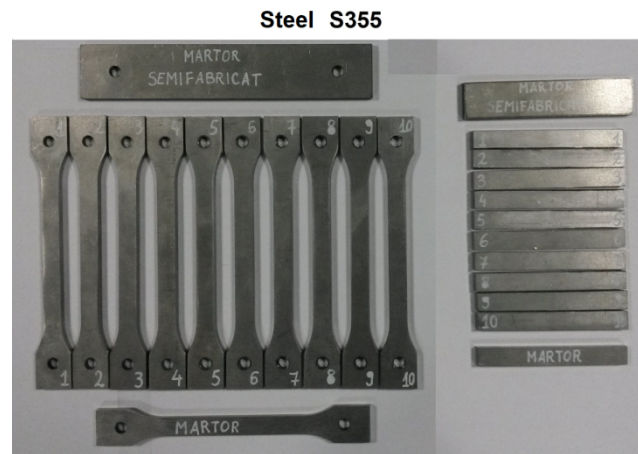
Figure 6. Tensile and bending specimens, made of steel.
