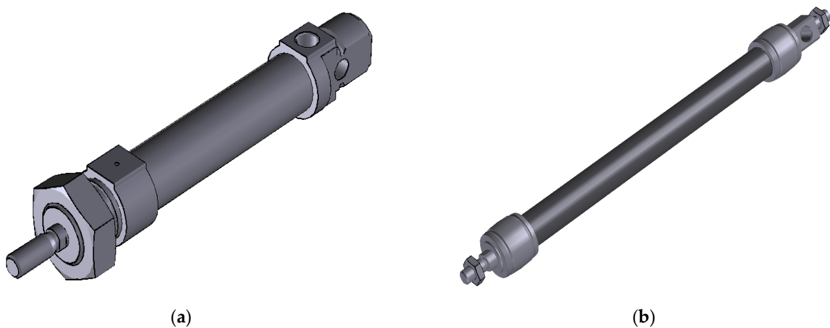
Figure 2. Studied pneumatic motors: (a) Single-acting cylinder (ESNU) [34]; (b) Pneumatic muscle (DMSP) [35].
