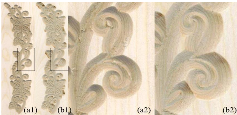
Figure 6. Router milling of Model 2: (a1) – Engrave 90°; (a2) – Detail for Engrave 90°; (b1) – Engrave 120°; (b2) – Detail for Engrave 120°.
