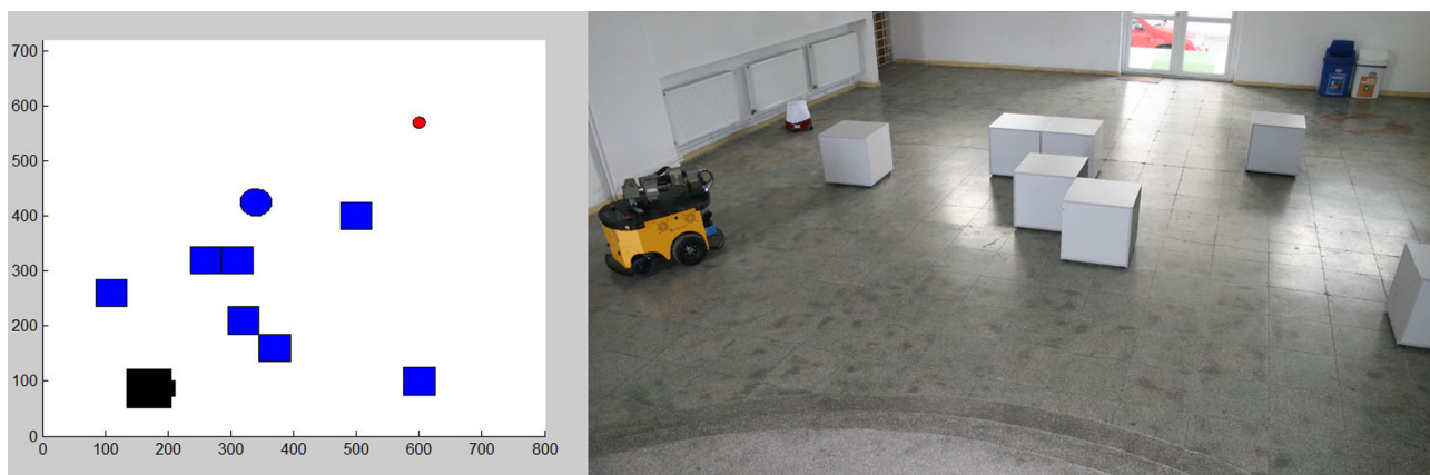
Fig. 5. A 7 m \times 8 m workspace with a robot, 7 fixed obstacles, 1 dynamic obstacle and a target.
