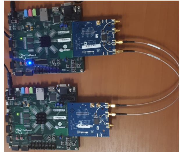
FIGURE 8. Experimental setup – Back-to-back “Zedboards” with FMCOMMSx AD daughterboards.
