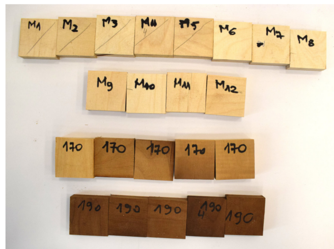
Figure 11. Images of control and torrefied poplar PW samples at 170 °C and 190 °C.
