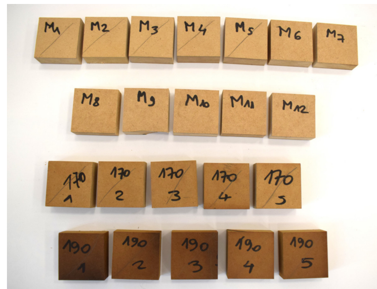
Figure 12. Images of control and torrefied MDF samples at 170 °C and 190 °C.
