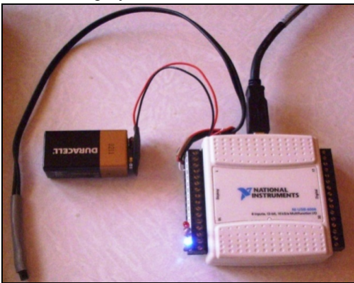
Figure 2. Simple and cost-effective proof-of-concept configuration: NI USB-6008 with red/blue LEDs (the second one lights, closing the Twitter loop by notifying an inferior temperature); LM35 sensor; 9V battery
