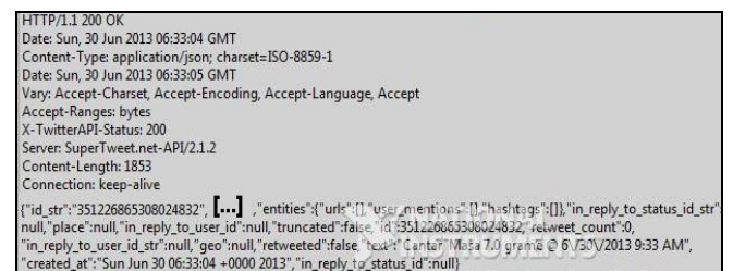
Figure 3 (b). HTTP Answer - fragments separated by [...] - in the case of SuperTweet Update Status.vi based on JSON
