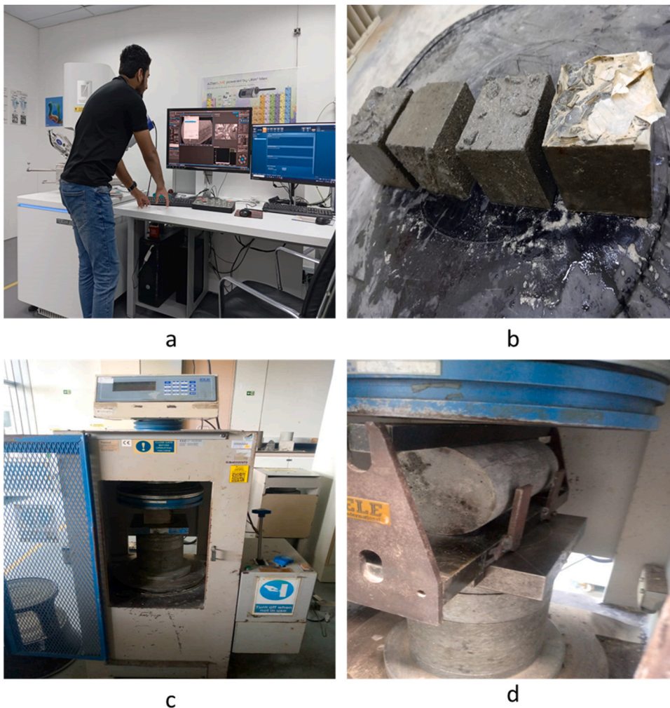
Fig. 2. (a) SEM of carbon fiber, (b) cured samples, (c) compressive strength testing (d) split tensile strength testing.
