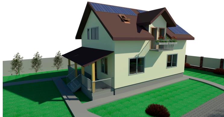
Figure 11. The case study building Revit model used for quantities assessment and thermal loads pre-calculations.
