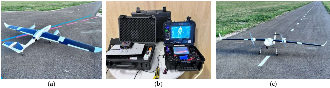
Figure 19. Ground testing of flight controls on the takeoff-landing runway: (a) motors testing; (b) thermal module testing; (c) preparation and verification of ground taxiing for the UAV model.
