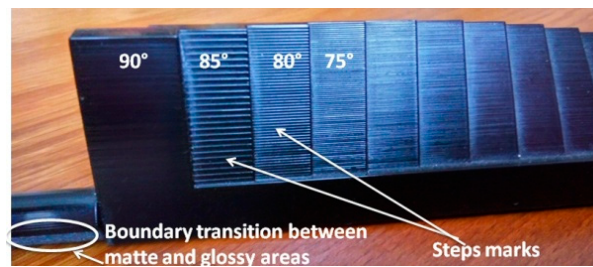
Figure 13. Flaws for samples printed in glossy style involve steps marks and a boundary transition between matte and glossy areas.
