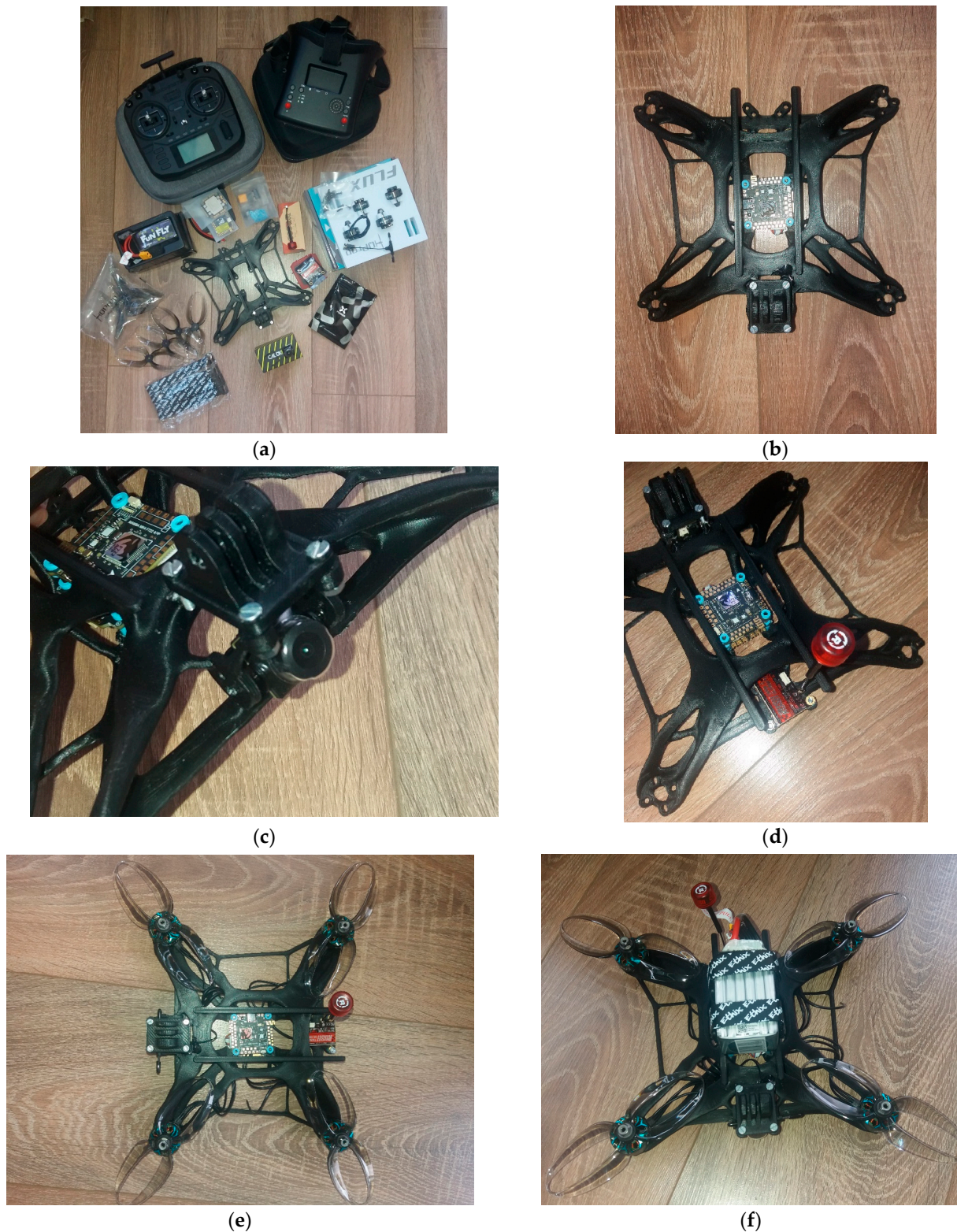
Figure 9. Stages of the quadcopter drone assembly process: (a) drone components; (b) mounting the FC and ESC in the central area of the frame; (c) mounting the FPV camera; (d) mounting the video transmitter and associated antenna; (e) mounting the motors and propellers; (f) mounting the battery.
