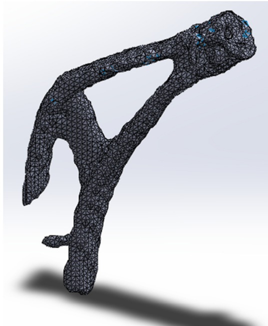
Fig. 4. TruForm-generated optimized femoral stem.
