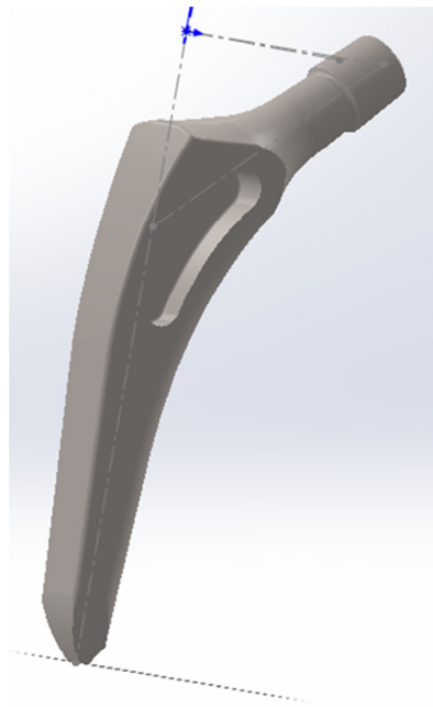
Fig. 5. Weight optimized femoral stem
